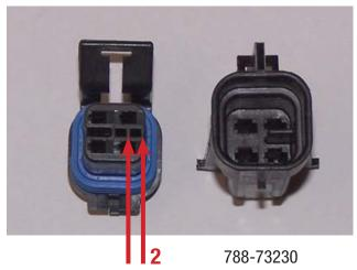
To make the square gray male connector work with the black square female connector cut the web indicated by arrow number 1. To make the square black male connector work with the female square gray connector, cut the two webs located at arrow 2, do not cut the center web.
