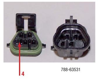
To make the trapezoidal gray male connector work with the black trapezoidal female connector cut the web indicated by arrow number 3. To make the trapezoidal black male connector work with the female trapezoidal gray connector, cut the two webs located at arrow 4.
