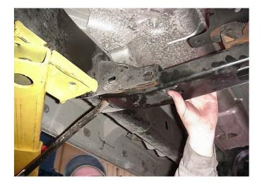
Pry the passenger side of the cross member down to aid in its removal.
