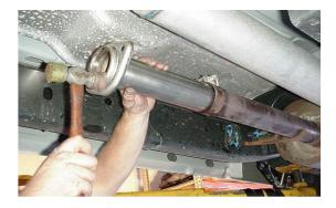
6. Carefully install the O2 sensors in the passenger side catalytic converter and the "Y"-pipe outlet as shown below. A small amount of anti-seize is recommended but **do not** get it on the sensor itself.
