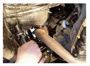
13. Before removing any cross member bolts, you must add a support to the transmission rear tail housing. Once supported, remove the 4 cross member bolts from the main frame brackets
