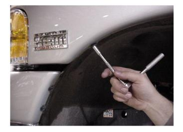
These screws need to be removed prior to removing both the LH and RH inner panels. This gives you lots of room to install your new headers. **Is that a Hemi behind those panels?**  6. Remove the LH and RH inner fender panels.
