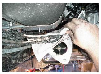
The reflective silver finish goes to the outside. Wrap the shielding material around the harness and fuel line and apply pressure to the Velcro strip. Warning – Do not run the vehicle without installing this thermal wrap \*
