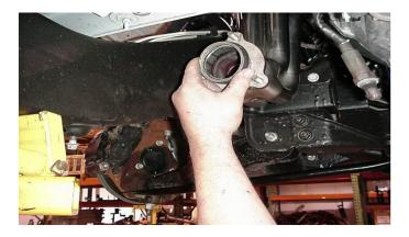
Install the sintered metal donut gaskets before you install the "Y"-pipe.
