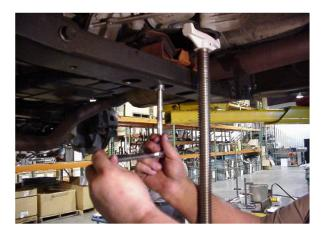
This shows the rear transmission housing support and removal of the transmission mounting bolt nuts.
