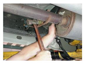
12. Loosen the nuts holding the "down tubes" to the cast manifolds .
