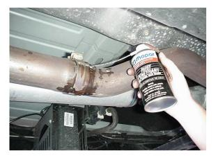
11. Loosen the muffler/"Y"-pipe clamp and separate the muffler from the "Y"pipe. You may need a dead blow hammer or a rubber mallet to accomplish this. Completely removing the muffler and tailpipe is not required but may help to eliminate interference while removing and installing your new header system.
