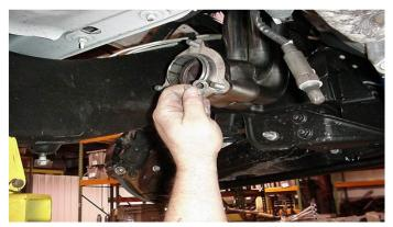
Install one spacer per stud. This prevents the gasket from being crushed beyond its intended yield point as the catalytic converters and "Y"-pipe are being tightened into position. ( Do this on both headers )
