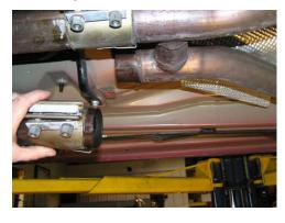
The "H"-pipe assembly should be completely free to remove at this point. Do this by lowering the rear of the
