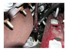
nuts and studs that you can get to from the top side of the engine at this time.
