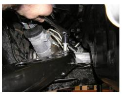
Slide the rack and pinion forward in the car enough to allow the upper steering shaft to slip out of the universal joint. Lay the steering shaft out of the way on top of the frame rail. Caution: Do not allow the steering wheel to rotate while the steering column intermediate shaft is disconnected – damage to the clock spring can result. If this occurs the clock spring must be removed and re-centered.
