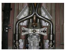
Reinstall the saved OEM band clamps over the stock tailpipe, raise the rear of the x-pipe assembly and slide the clamps over the x-pipe outlets. Make sure that the joint where the x-pipe outlets and the tails are joined, that the tubes are butted up as close as possible to one another by moving the x-pipe assembly back to meet the tailpipes.
