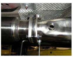
Assemble the "X"-pipe by slipping a band clamp over short leg of the X-pipe and inserting the left interim leg into the clamp. With x-pipe unit assembled slide a band clamp on each of the 2 inlet legs of the x-pipe and slide the whole assembly into the rubber hanger brackets and into the rear of both the left and right catalytic converters. Bend X-pipe hangers to aid alignment if needed.
