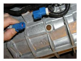
• Loosen and remove the 2 rear O2 sensors from the "H"-pipe. Be sure to mark the sensors so they can be put back in the same relative positions in the new system. The front right (passenger side) O2 sensor will have to be removed after the "H"-pipe is removed from the vehicle.
