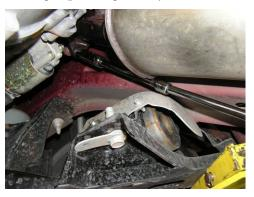
Remove the rear tailpipe couplers that were loosened in an earlier step by inserting the flat of a screwdriver
