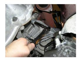
Now that the engine mounts are out of the way, the lower manifold nuts and studs can be removed. Do this on both the left and right sides of the engine. Remove the left (driver side) 02 sensor from the cast manifold utilizing the same precautions and procedures as the other sensors listed above. As all the nuts and studs are removed from the manifolds and block, lower the manifolds out of the engine bay. They will not be needed in your new system.
