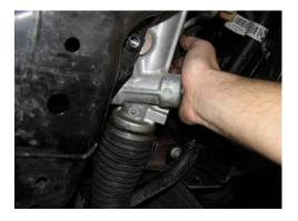
Install the steering shaft universal joint bolt and torque to 18 ft/lbs.
