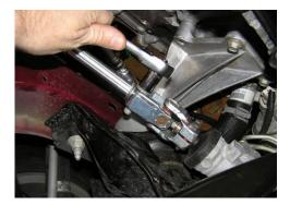
Loosen and remove the bolt holding the upper steering shaft section into the universal joint.
