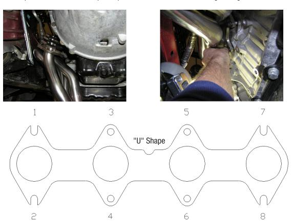
Use this torque chart for both the left and right header flanges.
