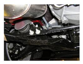
Begin the under – vehicle procedures by loosening the band clamps securing the "H"-pipe to the tail pipes. Do not remove the clamps at this time.
