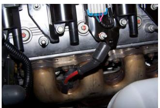
• After the spark plug wires have been removed, start removal of the left (driver) side stock manifold by loosening and removing the six (6) manifold bolts. The manifold must be removed from the bottom side of the vehicle. Either remove the spark plugs or use extra care not to damage them during the removal process. The engine bay should look similar to the picture to the right after the manifold is removed.
