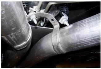
Move forward in the vehicle and loosen and remove the two (2) bolts and the two (2) studs holding the interim tube assembly to the back of the catalytic converter/tube assembly.
