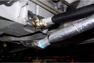
Note: The Chevrolet Service Instructions indicate that the O-ring seals on the end of the oil sump lines should be replaced anytime the lines are removed. These are a dealer only part and often must be ordered ahead of time. Please plan accordingly.
