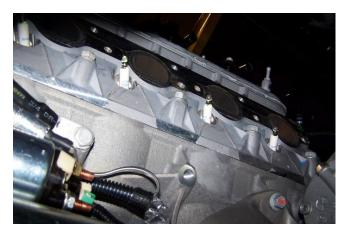
This should complete the removal of the stock system. Make sure that the motor mount nuts have been re-installed and properly tightened.
